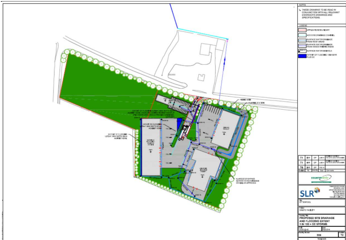
Drawing number 008 T2: Proposed Site Drainage and Flooding Extent 1 in 100 + CC Storms
